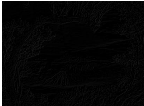
Figure 8. Image Convolution Results using Sobel filters
